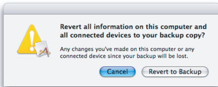
Figure 13-30 A customized alert showing the caution icon badged with an application icon
